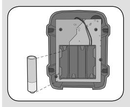
Install 4 AA Alkaline batteries (not provided). (Lithium batteries recommended for colder environments.) Keypad will beep.
