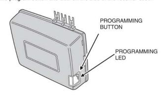
STEP 5 Program receiver. Momentarily press the receiver's program button. The red programming LED will light if there's room in the receiver's memory for another transmitter (40 maximum per receiver). The LED stays on for about 5 seconds. A transmitter must be entered while the LED is on. Press the desired transmitter button. The LED will flicker indicating that the receiver has accepted the transmitter.
