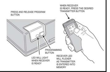
STEP 6 Add additional transmitters. Repeat Step 5 for each transmitter used with this receiver. Be sure to press the receiver's program button each time a new transmitter or a different transmitter button on a multi-button transmitter is pressed. If the LED doesn't come on when the receiver's program button is pressed, the receiver's memory is full (40 transmitters total). Use the erase function (Info 1) to remove ALL previously learned transmitters from the receiver's memory.
