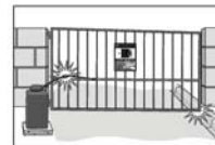
The gate hits the driveway, curb or other, and gets stuck or bent in an awkward position. (Swing Only)
