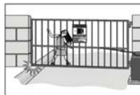
A foreign object is on the gate frame while the gate is moving. (Swing Only)
