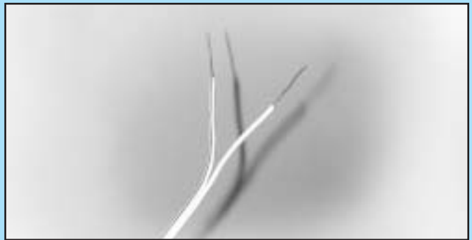
FIG. 3-6 Splitting and stripping.
