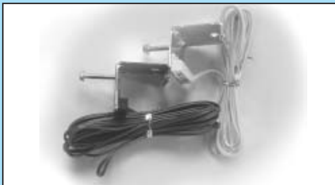
FIG. 1-10 Identify limit switches / insert set screws.
