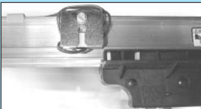
FIG. 7-3 Align "CLOSE" limit switch.
