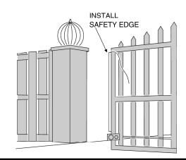
**STEP 6** Attach Cable. Attach safety edge cable to terminals as shown. Tighten cable grip assembly using pliers to assure a water tight seal.
