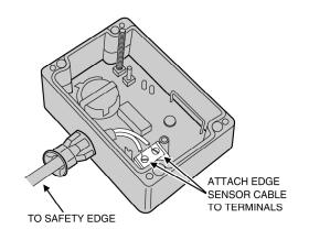
**STEP 7 Set Jumper.** Remove the battery protection strip. The MGT monitors the edge sensor for short circuits and cut wiring by measuring the edge sensor capacitance value. This function works with edge sensors such as Miller Edge Models MGR20 and MGS20. Some edge sensors may not present enough capacitance to pass this test. If a constant loop trouble condition is being indicated the test can be disabled by setting the Open Loop Test Option Jumper to the OFF position.
