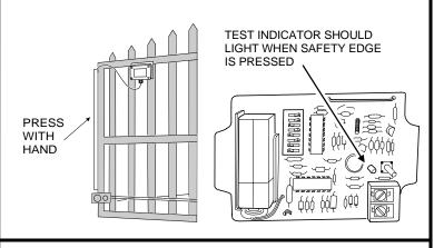
STEP 10 Test System. Activate the gate to close. As the gate is closing, press the safety edge with your hand. Gate should stop and reverse.
