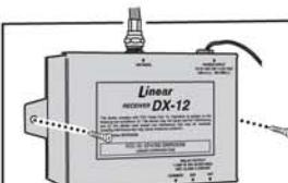
USE APPROPRIATE FASTENERS TO SECURE THE RECEIVER TO THE MOUNTING SURFACE
