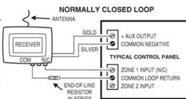
USE EITHER THE NORMALLY OPEN OR THE NORMALLY CLOSED TERMINAL AND THE COMMON TERMINAL
