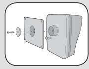
Connect PIR Motion Sensor box to mounting plate with silver screw. Tighten screw until PIR Motion Sensor stays in place when repositioned.
