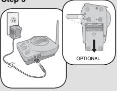
Plug in Base Station. Adhere rubber pads to bottom. 4 AA Alkaline batteries (not provided) are optional in case of power failures.
