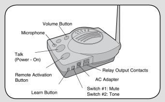
**Intercom Feature:** When PIR Motion Sensor has detected motion, the Base Station will allow you to listen through the PIR Motion Sensor for 10 seconds. If you wish to talk to the person on the other end, hold down the Talk button and speak, releasing it to hear.
