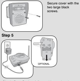
Plug in Base Station. Adhere rubber pads to bottom. 4 AA Alkaline batteries (not provided) are optional in case of power failures.
