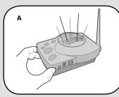
A Ensure that Base Station and PIR Motion Sensor are in close proximity to each other. Press and release learn button on Base Station. Buzzer will sound.
