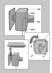
**Vehicle Alert Installation:** For cars, the best mounting position is about 4 feet high, between 10-20 feet back, and angled to see the back of car after passing the sensor.
