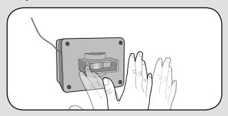
Test PIR Motion Sensor by waving hand in front of sensor. Test light should flash and the Base Station will buzz.
