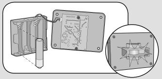
Install 4 AA Alkaline batteries. (Lithium batteries recommended for colder environments.) Test light will flash.
