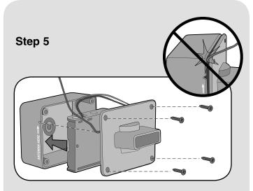
Insert battery pack facing away from circuit board and fasten cover with the smallest screws (provided). **NOTE:** Ensure the batteries do not touch the circuit board and the antenna and battery wires are not pinched.
