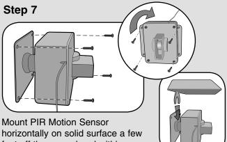
horizontally on solid surface a few feet off the ground and within 1/2 mile of Base Station (rotate sensor to access screw holes). Unit should be able to swivel as needed. Attach sun/rain shield.
