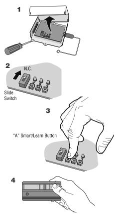
Repeat the steps 3-4 above with the yellow button on the remote control and the receiver Smart/Learn button "B" to program the CLOSE mode; and again with the green button on the remote control and the receiver Smart/Learn button "C" to program the OPEN mode.
