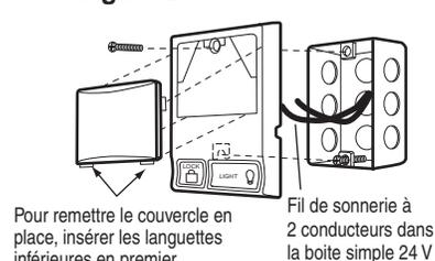
Figure 3 PANNEAU COMMANDE DE PORTE (ARRIÈRE)
