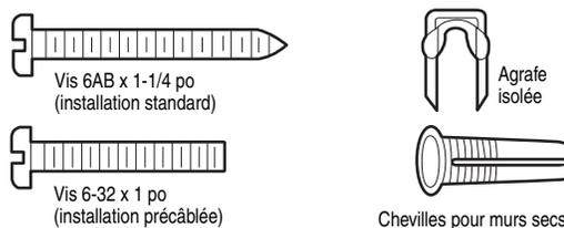
Figure 1 INSTALLATION STANDARD
