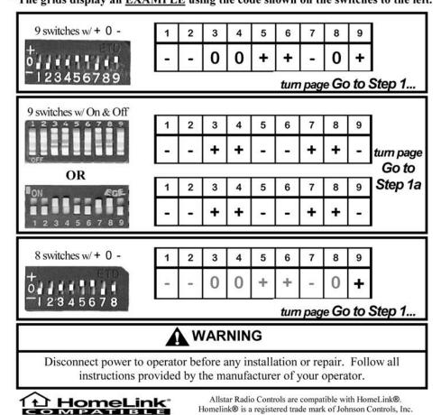
**NOTE:** The table has a row for each one of the three buttons since it is possible to set a unique code for each button. Write the code that you matched from your transmitter or receiver in the grids below.
