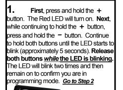
**1**a. First, press and hold the button. The Red LED will turn on. Next, while continuing to hold the - button, press and hold the + button. Continue to hold both buttons until the LED starts to blink (approximately 5 seconds). **Release** both buttons *while* the LED is blinking. The LED will blink two times and then remain on to confirm you are in programming mode. Go to Step 2
