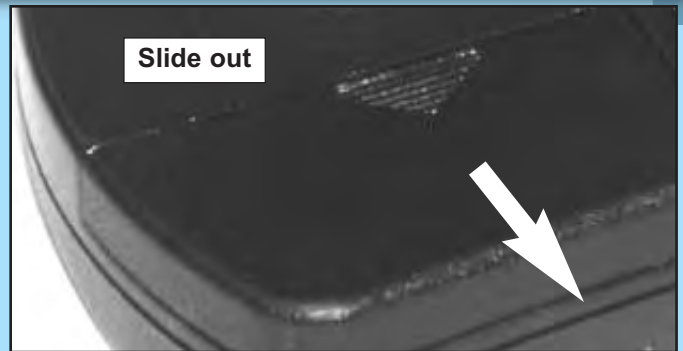
FIG. 8-1 Open battery cover.
