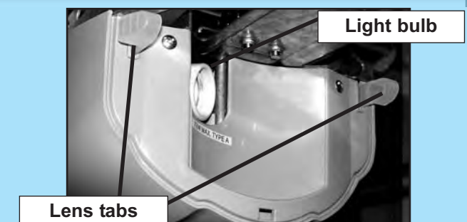
FIG. 9-1 Slide lens onto motor cover.
