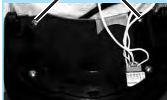
FIG. 5-2 Remove motor cover.
