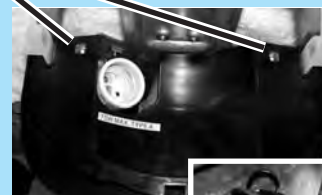
FIG. 5-3 Power cord strain relief.
